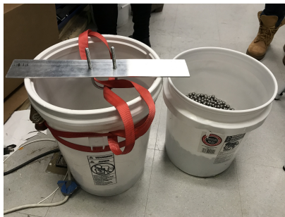
Fig. 7 Ball Bearings Transferred to Empty Bucket Suspended from Bridge for Testing
