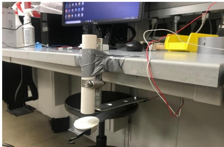
Figure 6: Configuration of Breath Force Meter for Calibration
